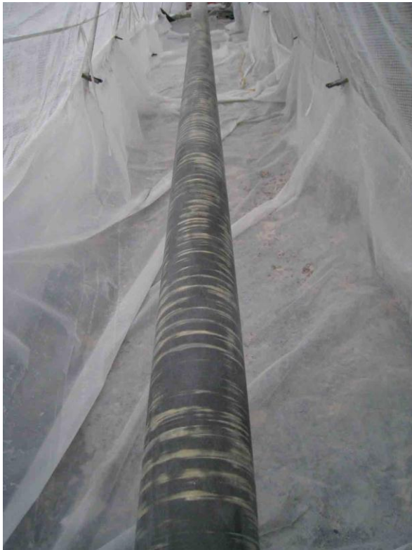
Photos 6 & 7. The mast ground down through most of the gelcoat to the glass, but not all the way through. The glass sock put on. This owner used a tube fabric from Giant Leap Rocketry: http://giantleaprocketry.com/products/components_composites.aspx .
