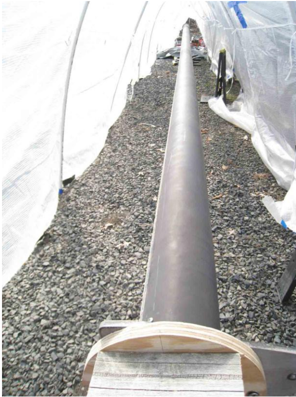
Photos 4 & 5. A fore mast set up horizontally under a temporary tent, supported by an engine repair crane.
