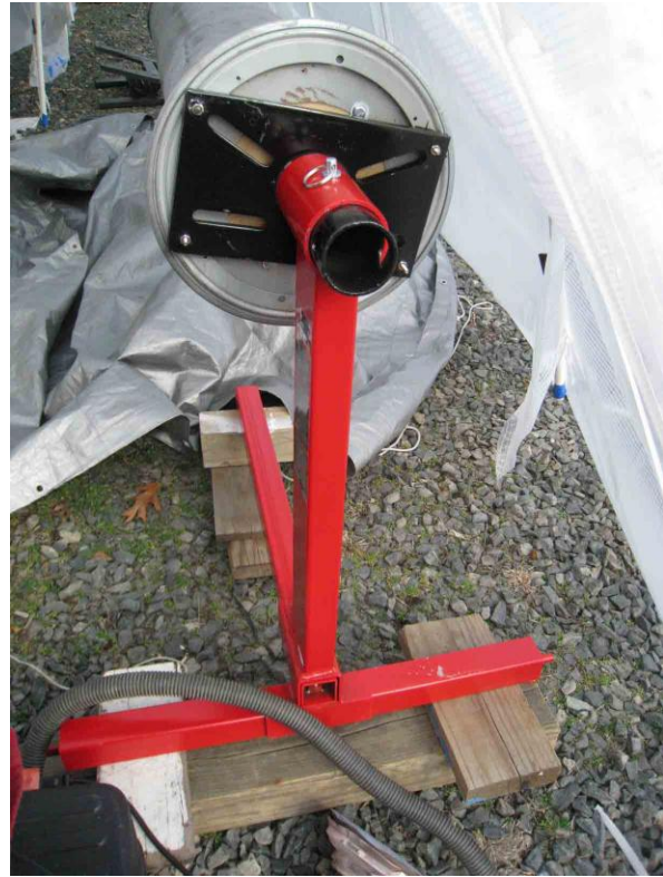
Photos 4 & 5. A fore mast set up horizontally under a temporary tent, supported by an engine repair crane.
