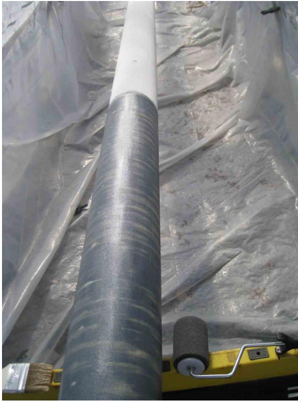
Photos 8 & 9. Wetting out the glass with epoxy, with a close-up of the lay-up. This owner bought epoxy from Progressive Composites: http://www.epoxyproducts.com/ .
