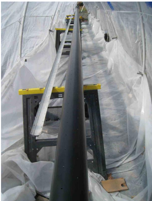
Photos 10 & 11. Painting and installation back on board. The paint was a moisture-cured polyurethane from: http://www.por15.com/CHASSIS-COAT-BLACK/productinfo/CHG/ .
