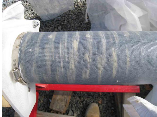
Photos 8 & 9. Wetting out the glass with epoxy, with a close-up of the lay-up. This owner bought epoxy from Progressive Composites: http://www.epoxyproducts.com/ .
